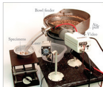
Figure 1. Proof-of-concept prototype automated micro-fossil picker. The feeder bowl guides matrix under the laser; the video camera detects size and brightness; fluorescing fossils are selected for further investigation using a puff of compressed air.
